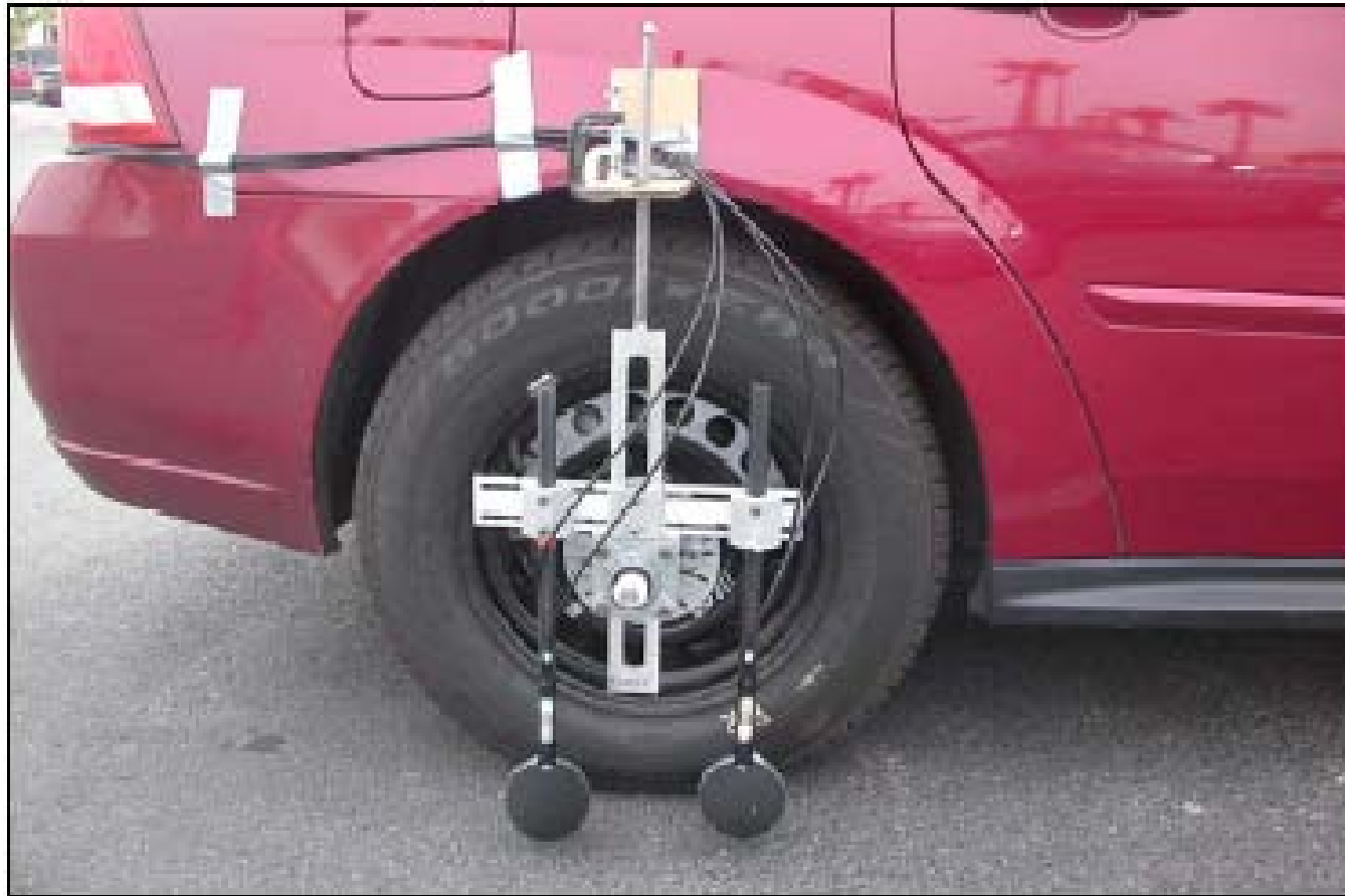
Figure 3: OBSI Equipment Installed on the Malibu Test Vehicle
